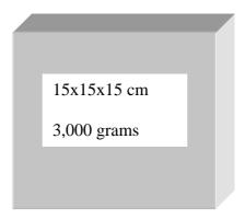
Material: Solidificated oil sludge added 20% (w/w) cement powder,
